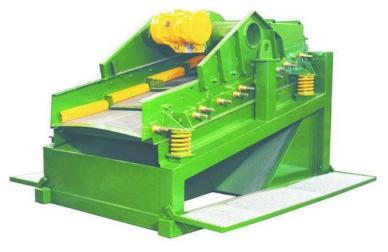
The shaker is mounted on a heavy duty square hollow section frame into which is built a tapered underflow chute that is used to direct the screened fluids towards a centrally located outlet. There is a mud feed header box sited at the rear of the shaker and the unit has a fold-down access platform on each side of the main frame.
