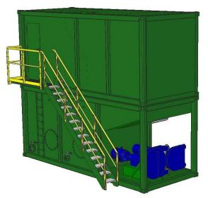
discharges the granular electrolyte under gravity directly into the electrolyte mixing tank. The control panel and pump inverters are located in the feeder unit. It has a 12m<sup>3</sup> built in water tank and forms a standard 20 foot container sized module, complete with ISO corner castings, for transport.
