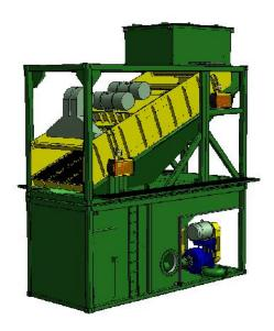
The SD2400DP Primary Shaker is a high capacity, steeply declined, single deck, linear motion shaker with up to 4 No. Metso MM200 centrifugal discharge pumps. The unit is used for the primary separation of gravels, coarse particles or clay balls. The SD2400DP consists of a shaker module mounted on top of a 20' container sized pump tank module plus two free-standing discharge pumps.
