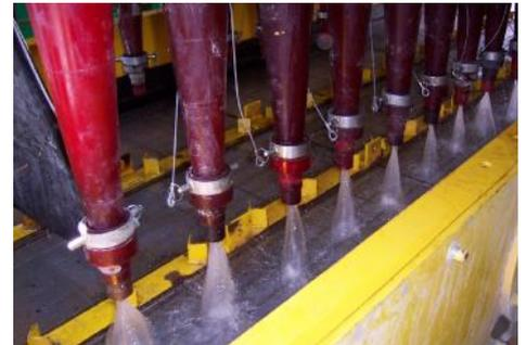
The SOLIDSMASTER® 400DP can be used on its own, downstream of a primary screen such as an SD600 or a DD800 or upstream of desilters such as SU8DP, SU10DP or SU72DP. The rate of solids removal from the SOLIDSMASTER® 400DP is governed by the characteristics of the dirty mud but can be up to 100 tonnes/hour.
