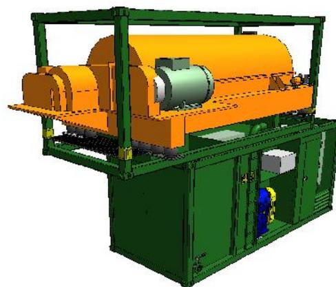
The centrifuge module has a heavy duty hollow section frame in which the centrifuge, the bowl drive motor, the scroll drive motor, the oil cooler and the fluid feed pipe are mounted. A solids discharge chute with retractable diverter plate and centrate discharge pipe is built in to the centrifuge module. Normally the separated solids would discharge on to the ground, for removal by back-hoe or front-end loader or on to a conveyor for transport to a storage area.
