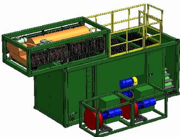
The centrifuge and its motors are mounted on a heavy-duty hollow section steel frame measuring 4000 x 1800 x 1190 mm high. The inverters, electrical controls, touch screen PLC, inverter controlled discharge pump and centrate collection tank are all housed in the Powerhouse Module, which also incorporates a staircase for access to the upper level.
